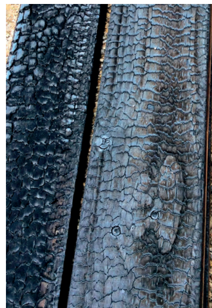
The Douglas fir planks after charring
