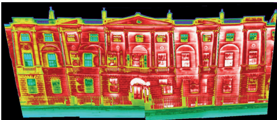
Thermal image composition showing heat loss from Bute House, Edinburgh (Image: Kal Murray, Eco Surveys)
