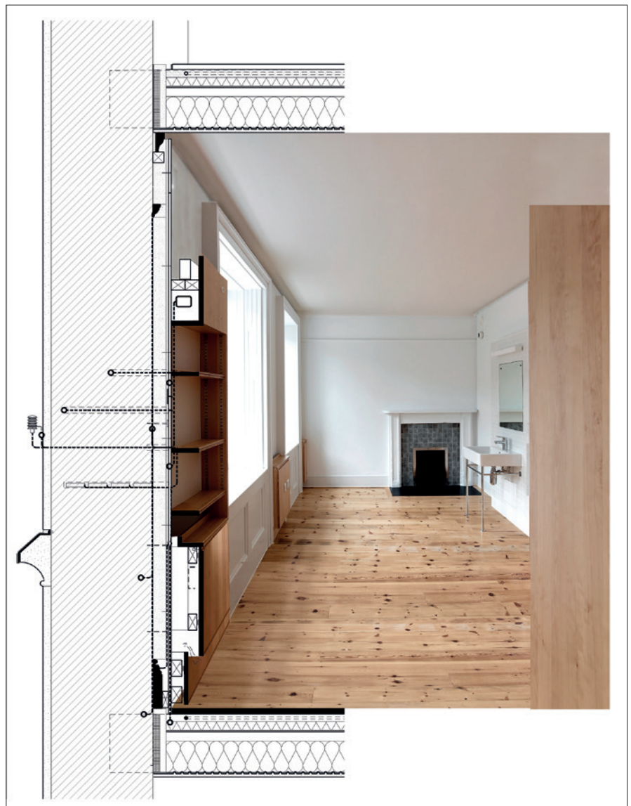
Computer modelling indicated that the cooling effect of a 60mm-lining of vapour permeable insulation would not cause an unacceptable increase in moisture in the masonry, but long-term monitoring was essential. The diagram shows an external weather station and probes installed at different depths in the masonry to monitor changes in temperature and relative humidity. (Image: 5th Studio)
