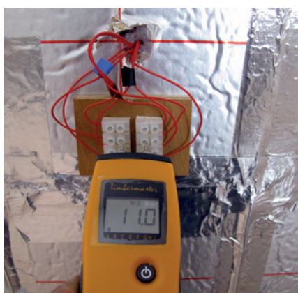
Measuring the moisture content of the dowels manually, using a resistance moisture meter. The dowels are connected to terminal blocks located to suit the spacing of the pins on the moisture meter. This enables repeated measurements to be made quickly and easily.
