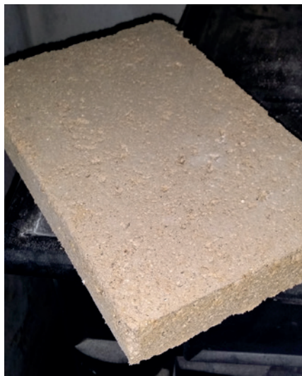
One of the pre-production insulation panels tested, 62mm (2½") thick
